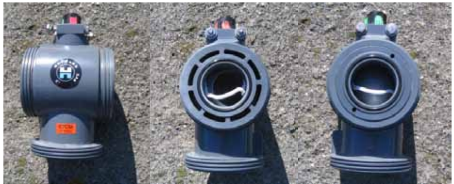
Fig. 4. Hayward valve that failed due to high heat.
